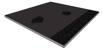
Rutting and Shoving. A depression or ripple of the pavement in the wheel path, it is a structural failure due to excessive loading of that pavement. It is a sign of an unstable asphalt pavement experiencing plastic flow. Pattern loss and movement will occur if StreetPrint is placed on this surface.
