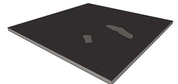
Bleeding / Flushing. Through the action of vehicle tires, heat and migration of excessive asphalt cement (AC) to the surface. Surface texture becomes filled with liquid AC, creating a weakened bond for the StreetBond coatings. This may indicate an excessive amount of AC in the mix.
